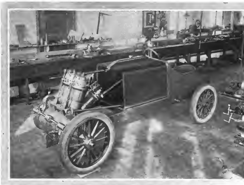
CHRISTIE RACER, SHOWING COMPACTNESS OF POWER PLANT.
